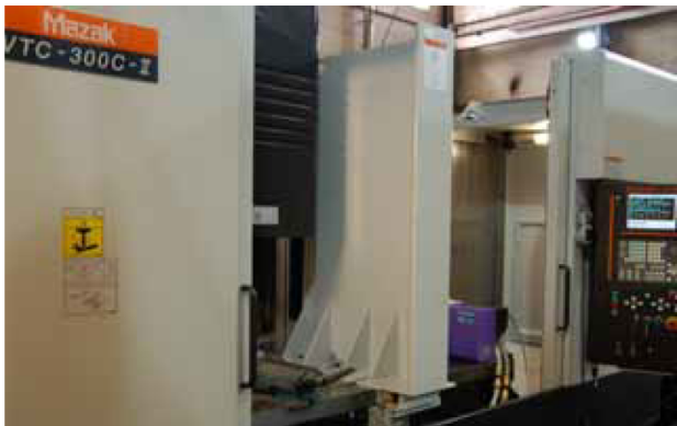
4-axis pendulum machining on Mazak-300C.II
