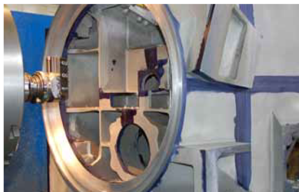
Horizontal boring with 5-axis DRO
